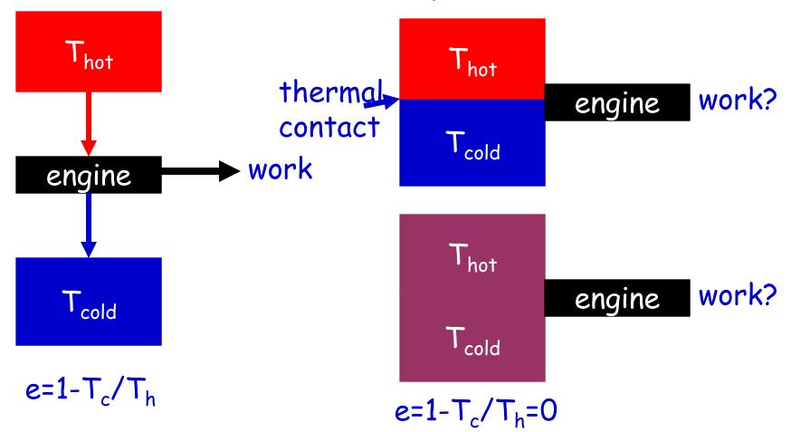
The transport of heat by conductance is irreversible and the engine ceases to work.
