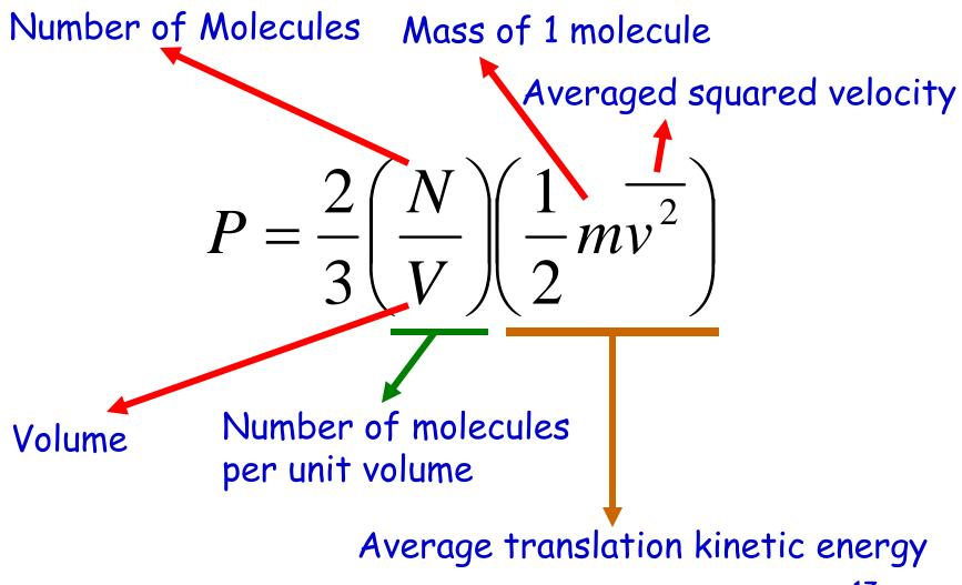
$$PV = \frac{2}{3}N\left(\frac{1}{2}m\overline{v^{2}}\right) \quad \text{Microscopic}$$
