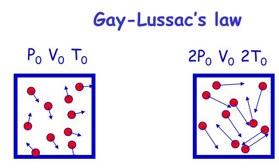
If, at constant volume, the temperature is increased, the pressure will increase by the same factor  $P \sim T$
