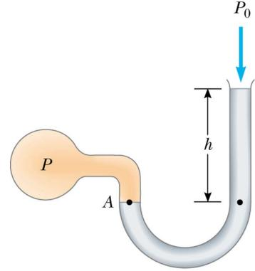
The open-tube manometer. The pressure at A and B is the same:  $P=P_0+\rho gh$ so  $h=(P-P_0)/(\rho g)$
