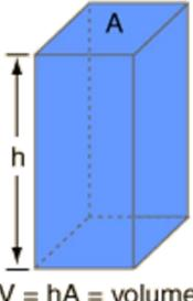
V = hA = volume weight = mg Static fluid pressure does <u>not</u> depend on the shape, total mass, or surface area of the liquid. Pressure =  $\frac{\text{weight}}{\text{area}} = \frac{\text{mg}}{\text{A}} = \frac{\rho \text{Vg}}{\text{A}} = \rho \text{gh}$
