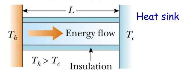
An insulated gold wire (i.e. no heat lost to the air) is at one end connected to a heat reservoir (T=100  $^{\circ}$ C) and at the other end connected to a heat sink (T=20  $^{\circ}$ C). If its length is 1m and P=200 W what is its cross section (A)?
