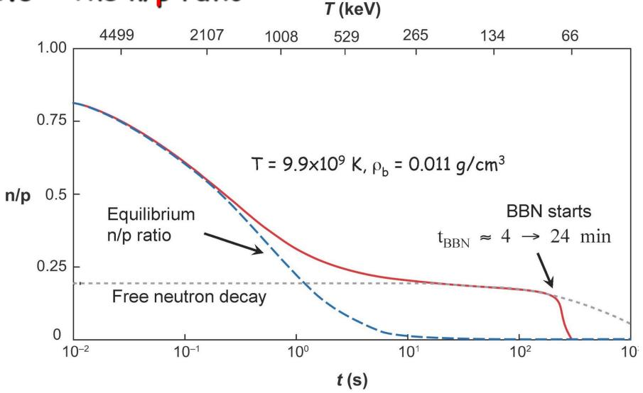
Neutron-to-proton (n/p) ratio as a function of time and temperature. The dashed curve is given by  $\exp(-\Delta m/k_BT)$ . The dotted curve is the free-neutron decay curve,  $\exp(-t/\tau_n)$ . The solid curve indicates the resulting n/p ratio as a combination of the two processes. BBN starts at  $t \sim 4$  min.
