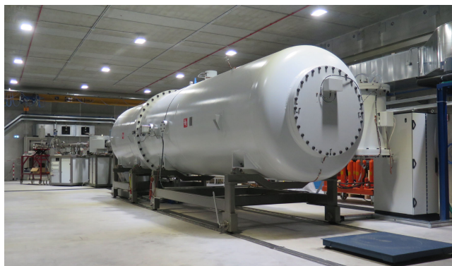
FIG. 13. Photo of the 3.5 MV Singletron accelerator recently installed at LNGS. From Matthias Junker.
