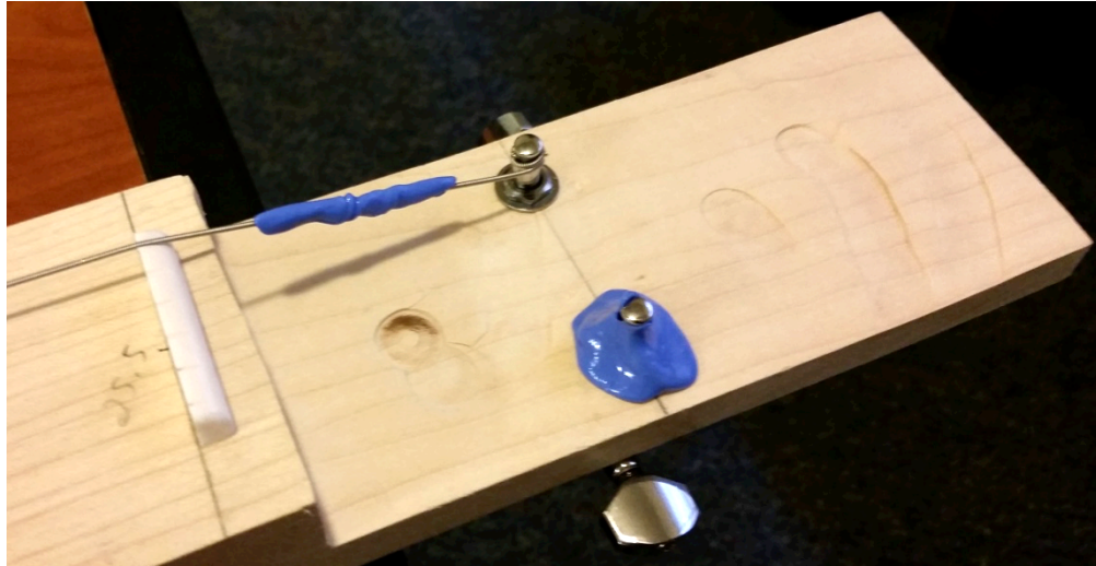
Picture 2 Tuning pegs and nut on the head of the guitar. Note the putty used to reduce vibration of the string behind the nut, as well as the other tuning peg.
