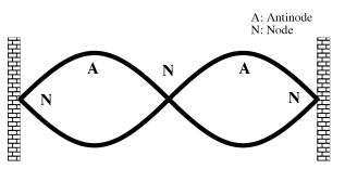
completely destructive. At other points, called **antinodes**, the waves reinforce one another so that the amplitude is largest here and the interference is said to be constructive. The standing wave is on a string that is fixed at both ends. The nodes, labeled "N" occur at the fixed ends and in the center at 1/2 the wavelength. The antinodes occur at "A."
