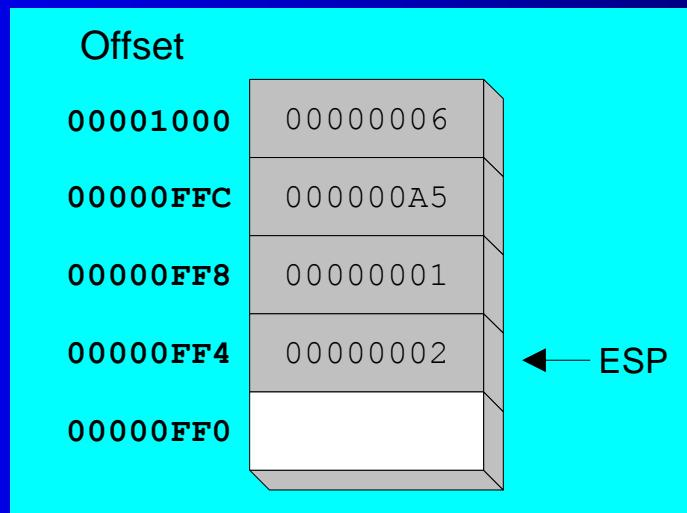
The stack grows downward. The area below ESP is always available (unless the stack has overflowed).
