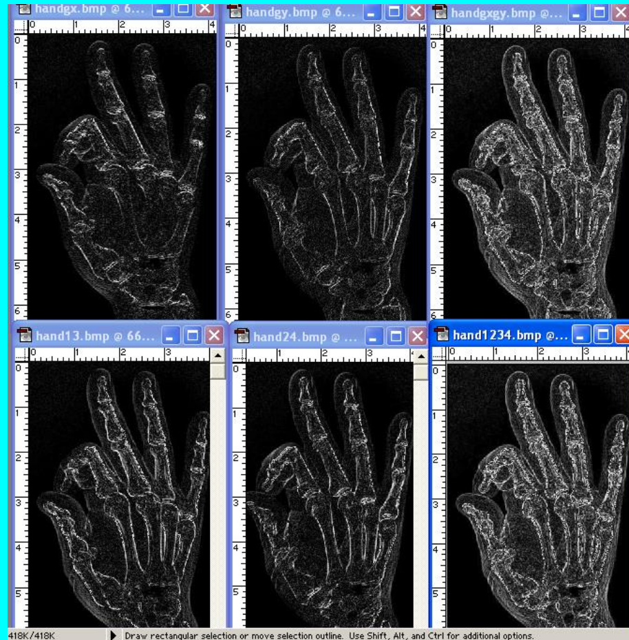
Figure11. Results obtained by employing different Gradient operators to an X-ray image of hand. The type of the operator is shown by the last two or four letters of the image title, give on the top of each image.
