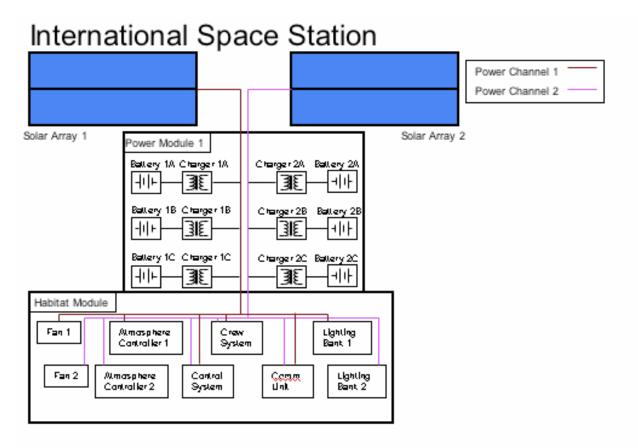
International Space Station Power Channel 1 Power Channel 2 Solar Array 1 Solar Array 2 Power Module 1 Battery 1A Charger 1A Charger 2A Battery 2A 3E BE Battery 18 Charger 18 Charger 28 Battery 28 Battery 10, Charger 10, Charger 20 Battery 20 36 **∃**E Habitat Module Command Module Fan 1 Almas phere Crew Lighting Fan O Lighting Main Controller 1 Beant S System Beint 1 Computer 1 Lighting Fan 2 Mmasphere Control Come Fan 4 Rabatic Main Cartraller 2 Unk. Bent 2 Workstation System Computer 2
