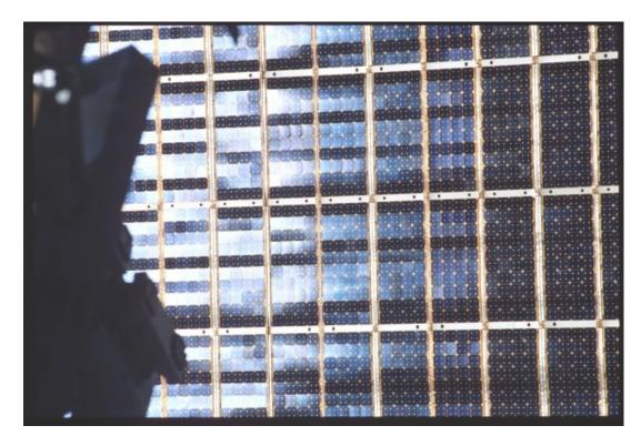
In this close up image of the solar arrays used on the ISS, you can see many individual panels. Each panel has a border of white. If you look closely at the image, you can see that there are 40 individual cells in a panel. The panel is four cells wide and 10 cells long.
