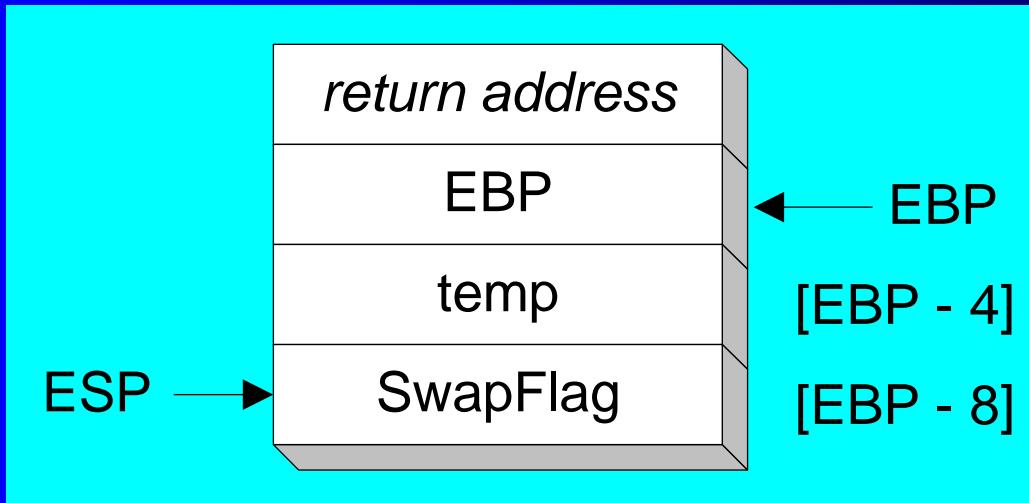
The ADD instruction adds -8 to ESP, moving it downward and creating an opening in the stack between ESP and EBP for the two local variables.
